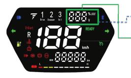
Voltage Of The Battery: This will be displayed on the speedometer when the ignition is turned on.
